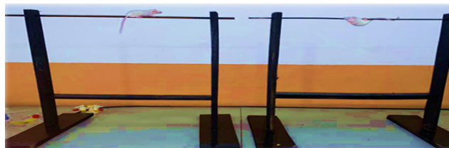
Figure 4: Two units of Beam (rod) walking test apparatuses with 2-mm and 4-mm iron rods
