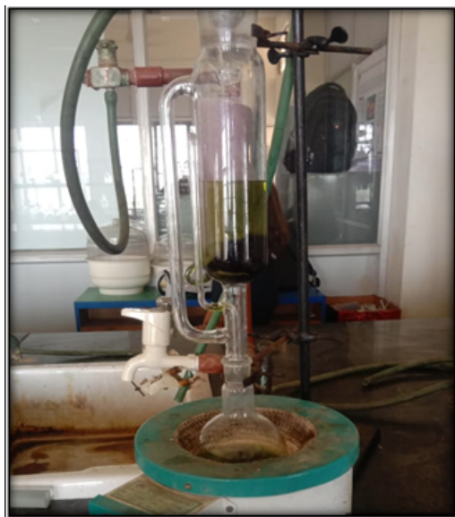
Figure 1: Soxhlet extraction of PBL
